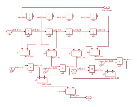
The fixed-point data types propagate through the subsystem. Inputs inherit the data types of the signals presented to them. Where required, internal rules of the blocks determine the output data type, given the input data types and the operation performed (for example, the Product blocks).
