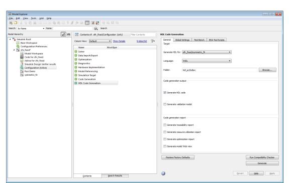
The following figure shows the top-level **HDL Code Generation** options pane in the Model Explorer.
