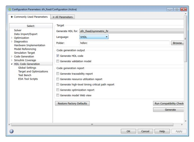
The **HDL Code Generation** pane contains top-level options and buttons that control the HDL code generation process. Several other categories of options are available under the **HDL Code** entry. This exercise uses a small subset of these options, leaving the others at their default settings.
